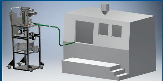
The VAC-U-MAX AM-MPRS is designed for safe and productive vacuum removal and sieving of Reactive and Non-Reactive Metal Powders as well as Polymer and Ceramic Powders.
